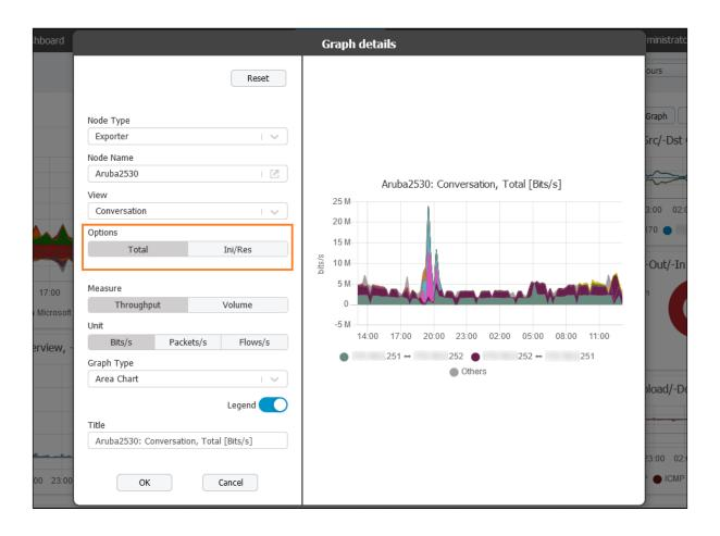
For example, if you want to monitor which conversations are consuming the most of your traffic, you can do that by observing **Total** distribution of traffic between Source (Src) and Destination (Dst) or by observing the aforementioned traffic distribution by opting for conversations between Initiators and Responders (Ini/Res).
