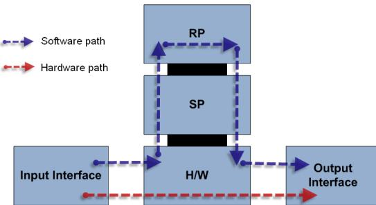
Figure above shows the concept of two paths for NetFlow packets, the hardware (red) and software (blue) paths and the configuration for each path. Normally on Cisco Catalyst 6500 Series Switch both hardware and software based NetFlow is configured.
