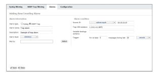
Screenshot above shows an example of an Alarm configuration. This Error level alarm will trigger if SNMP Trap message is sent from 10.10.10.10, with Trap OID 1.3.6.1.4.1.8072.
