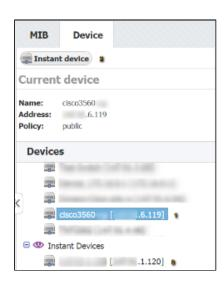
To select a device from the application database, simply select it from the DB devices list in the Device Tab (1). If the device you want is not in this list you can create it by going to > Settings > Control Panel > Devices. For more information go to article Configuring Devices.
