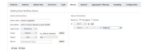
Screenshot above shows an example of threshold alarm. This alarms triggers if total traffic on interface Fa1 (link to Verizon) exceeds 800 Mbps. On alarm trigger an email will be sent to Super Administrator.
