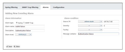
Screenshot above shows an example of an Alarm configuration. This alarm will trigger if syslog message is sent from 147.91.7.65, with severity level 3 and message containing Authentication failure.
